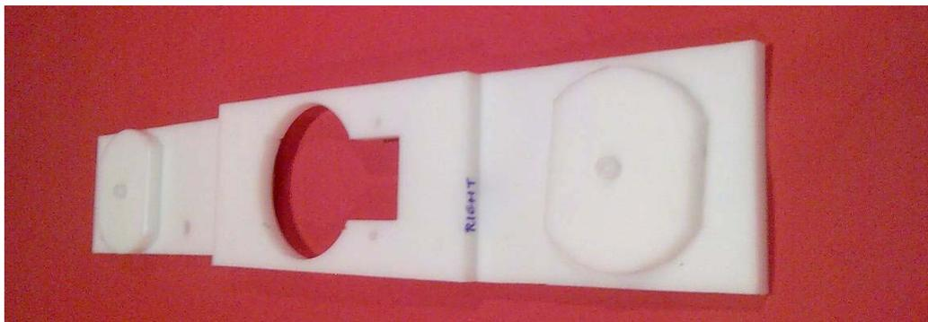
Figure 51. Extender panel for the wider beds to bridge the required gap between the two halves of the measurement wall.
