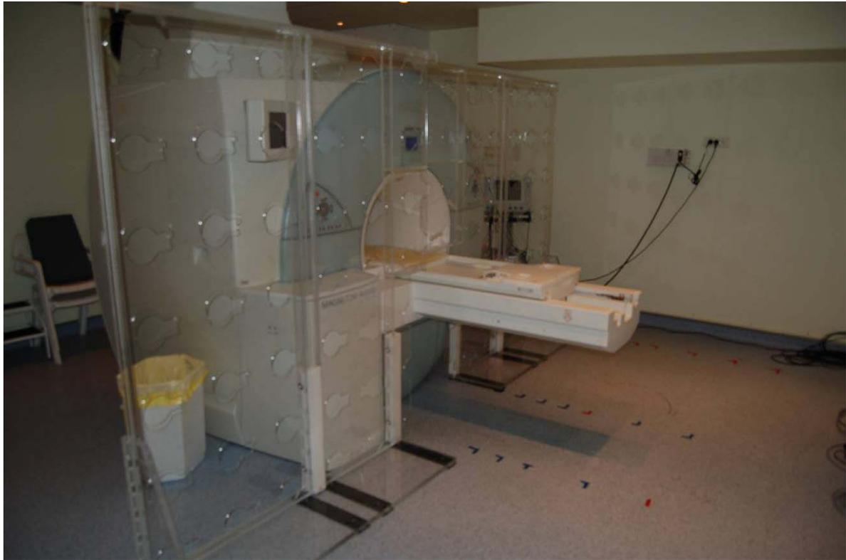
Figure 50. Cylindrical bore machine measurement grid, vertical plane defined by the wall, horizontal steps marked with tape on the floor.
